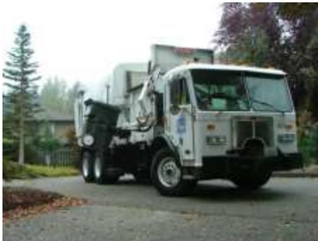
Figure 3: Automated side-load
