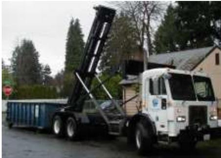
Figure 1: Tilt frame drop box “roll-off” truck
