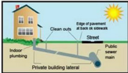
Gravity Sewer System
